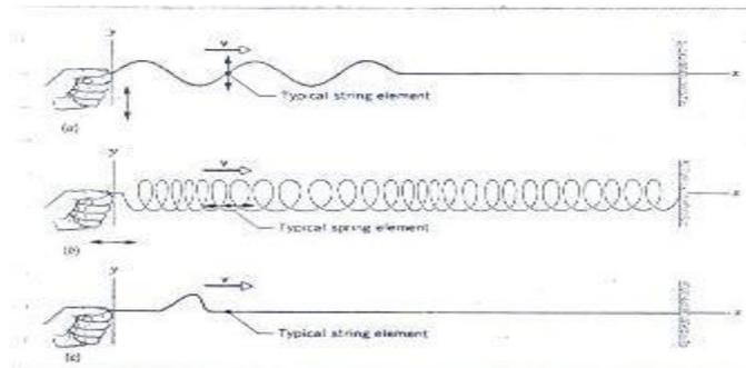
Figure 1 (a) Sending a transverse wave along a string. Each element of the string vibrates at right angles to the direction of propagation of the wave. (b) Sending a longitudinal wave along a spring. Each element of the spring vibrates parallel to the direction of propagation of the wave. (c) Sending a single transverse pulse along a string.
